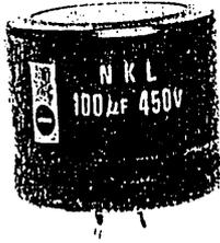
A range of general purpose aluminium electrolytic capacitors featuring extended temperature range for power supply applications. Electrical connections via PCB snap-in terminals on a unified 10mm pitch. Recommended PCB hole size 2mm diameter.
