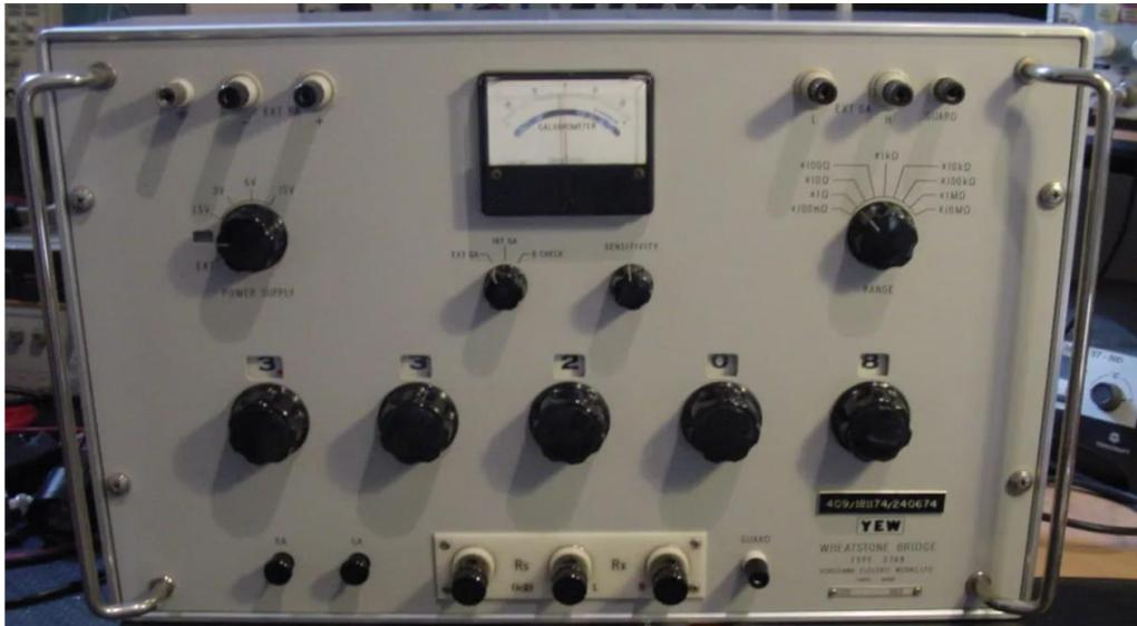
$$X = \frac{R_1}{R_2} R_3$$
